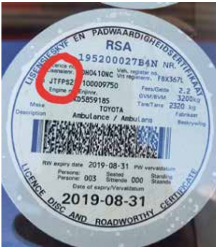
The licence disc says it is an ambulance but the P in the VIN number indicates it is actually a panel van
