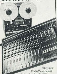
electronics gives totally professional results and offers a host of features such as: \* 4 Auxiliary sends \* Full 8 track routing \* 4 auxiliary returns with equalisation (giving 16 useable inputs and mixdown) \* Semi parametric equalisation \* 12 track monitoring \* Inserts on all 8 groups \* ½" tape - 15 ips tape speed \* Frequency response 40Hz-2Khz
