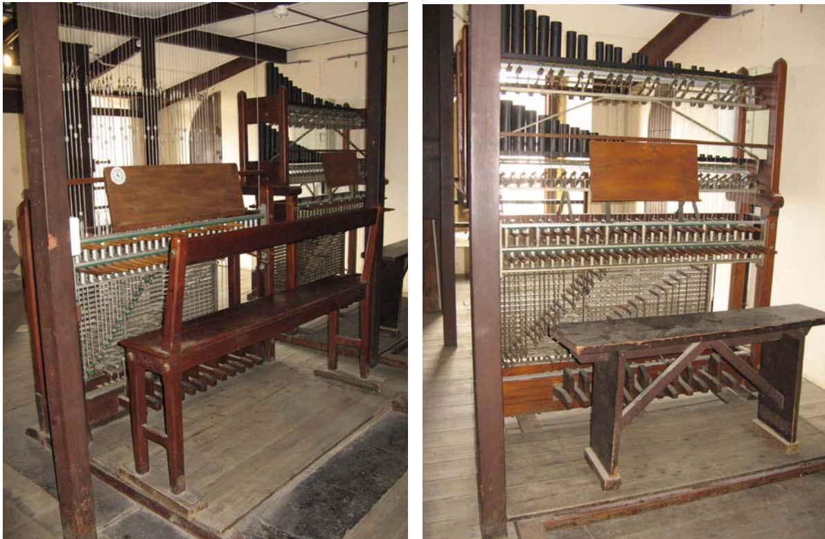
Figure 21: The two clavier are almost identical. The one on the right has lead pipes that produce the same tune as the other clavier but the sound can only be heard within the bell chamber.
